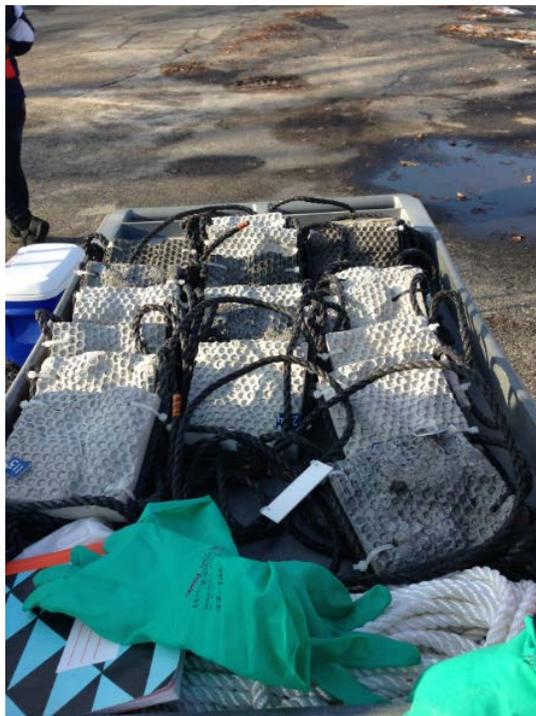
Figure 2- EONcrete tiles before deployment. The textured side is shown. The tiles vary in composition.
