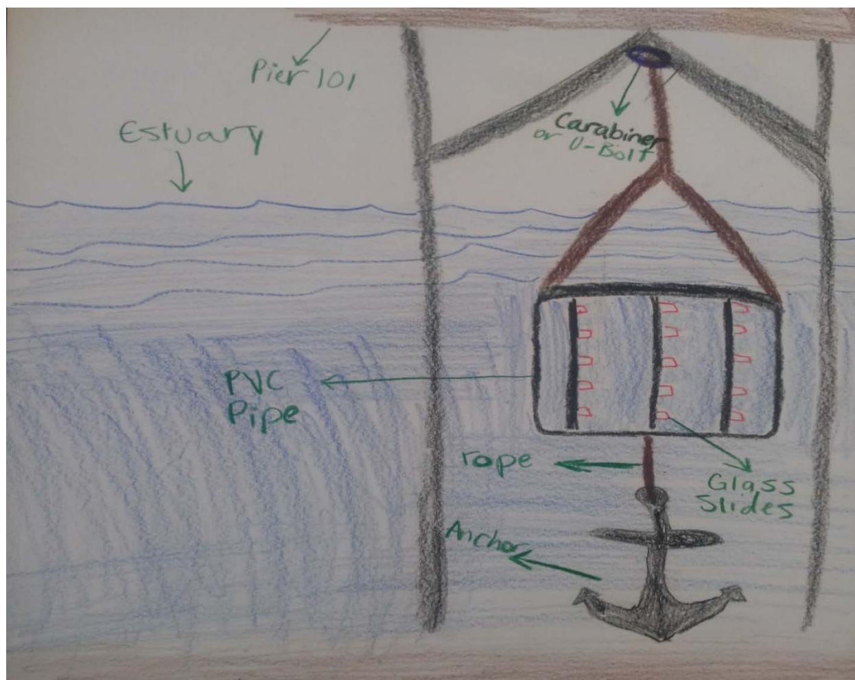
Figure 1 shows the design of the quadrat with the glass slides with the use of string, a PVC Pipe and an anchor in the Hudson River Estuary.
